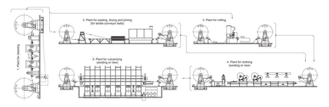
Purpose: Total regeneration of "rubber" conveyor belts. Main technical characteristics: Belth width (A): 1,6; 2,0; 2,4; 3,2. [m] Other: according to your request. We offer:
